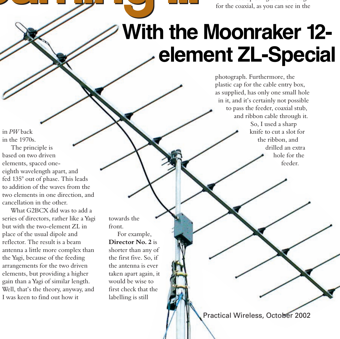
● Fig. 1: (Right) The Moonraker 12-element ZL-Special in use at G4HLX/P during the PW 144 MHz QRP Contest, June 2002 (see text).
